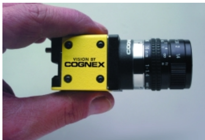
Cognex CDC Series cameras merge high-performance digital camera technology with low-cost CMOS image sensing, and are available in both large format and standard resolution models.
